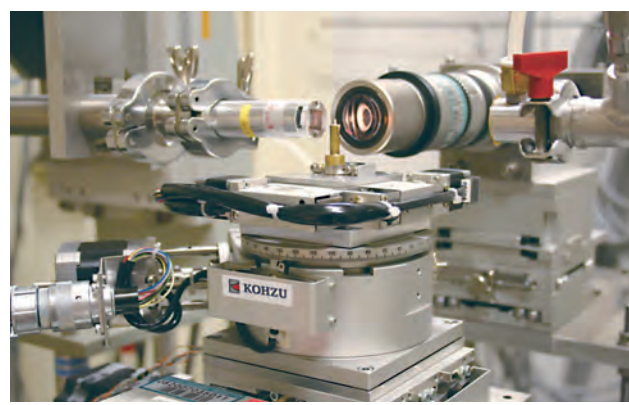
This Picture is shown as X-ray CT with SPU-1A for analysis of collected particle from Itokawa asteroid, Japanese Hayabusa mission (photo SPring-8).
