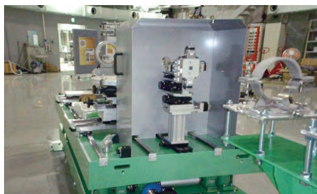
The slit is installed in a XAFS instrument.
